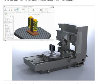
Enable digital manufacturing with PTC Creo suite of NC and Tooling extensions.
