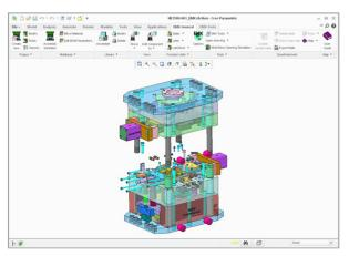
An exploded moldbase in PTC Creo Expert Moldbase Extension.
